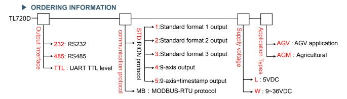
E.g:TL720D-232-STD1-L-AGV:RS232Output Interface/Standard format 1 output/5VDC/AGV application. Note: AGM does not currently have MODBUS protocol.
