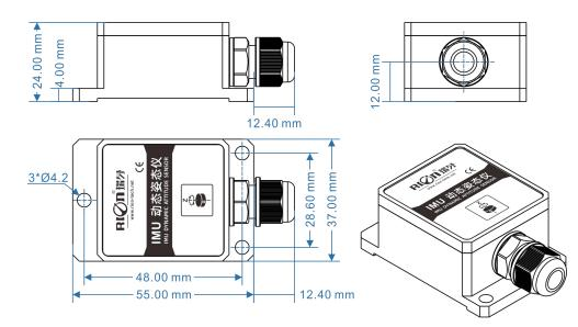
Shell size: L55×W37×H24mm Installation size: L48×W28.6×H24mm ounting screws: 3 M4 screws ▶ PRODUCT INSTALLATION DIRECTION
