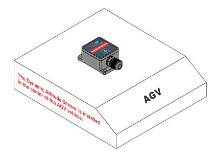
2. The installation of the instrument should be kept parallel to the surface of the measured object, and reduce the influence of the dynamic and acceleration on the angle meter. Incorrect installation will lead to measurement errors, with particular attention to "surface" and" line "
